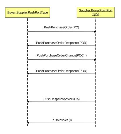
Figure 7: Direct Connect using Push model
