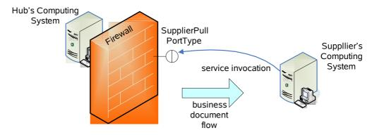
Figure 3: Supplier invokes "pull style" interface of Hub's Web Service
